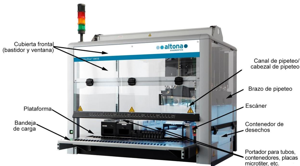
**Fig. 1: Instrumento AltoStar® AM16**
