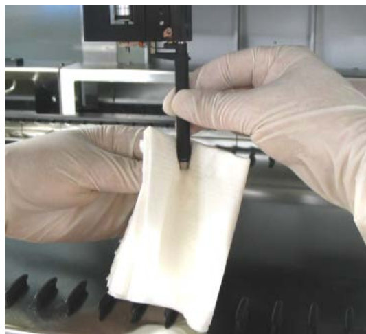
Fig. 23.: Cleaning the Stop Disk and O-Rings
