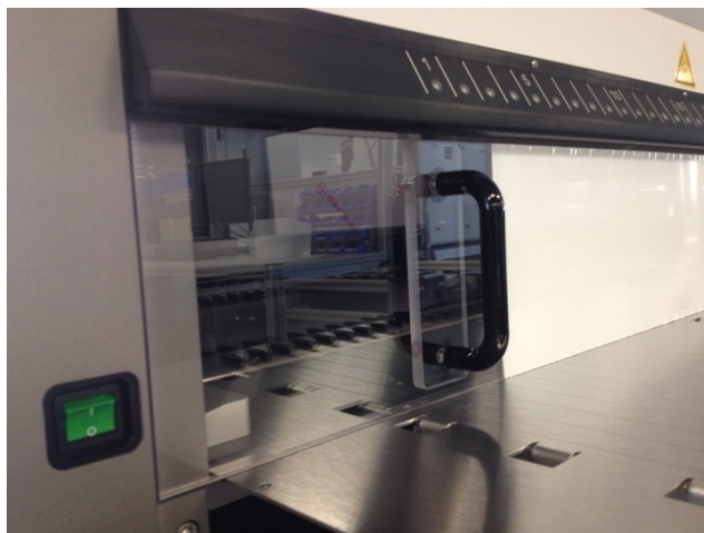
Fig. 24.: Mounting the UV Front Cover
