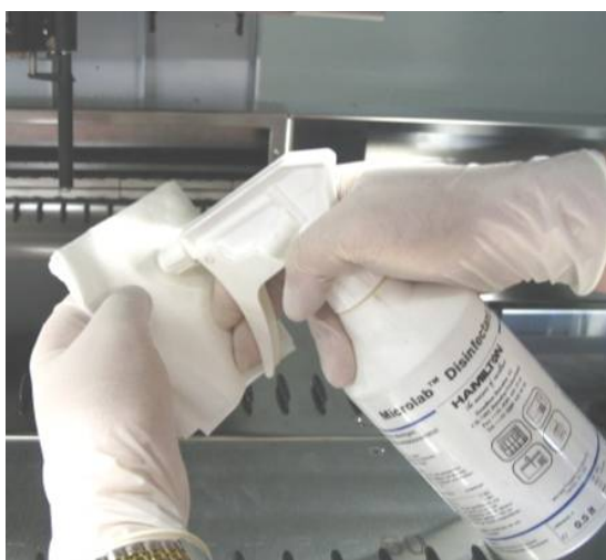
Fig. 22.: Cleaning the Tip Eject Sleeve
