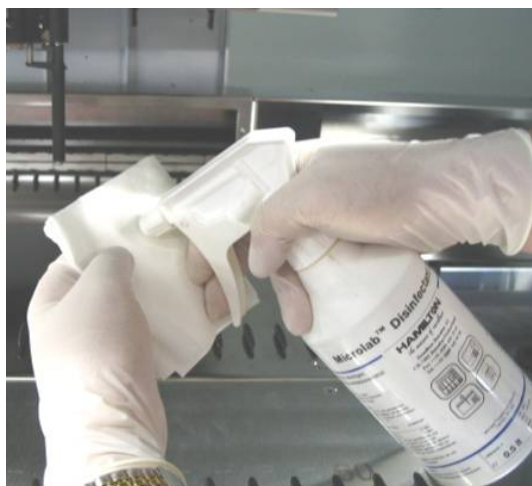
Fig. 23.: Cleaning the Stop Disk and O-Rings
